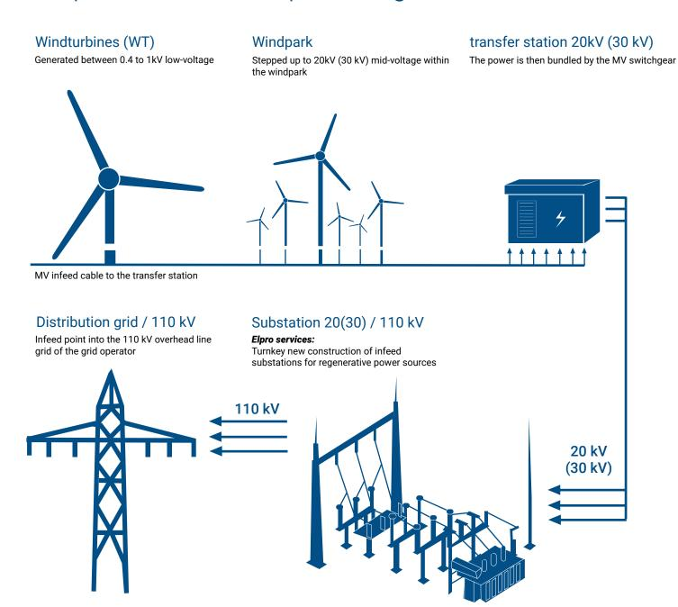
Windparks are the backbone of regenerative power conversion and consist of at least three wind turbines. The turbines used to convert wind energy into electrical power typically generate voltages of less than 1,000 VAC. Transformers that are usually arranged in the turbine towers convert the low-voltage into mid-voltage of 20,000 V or 30,000 V.
